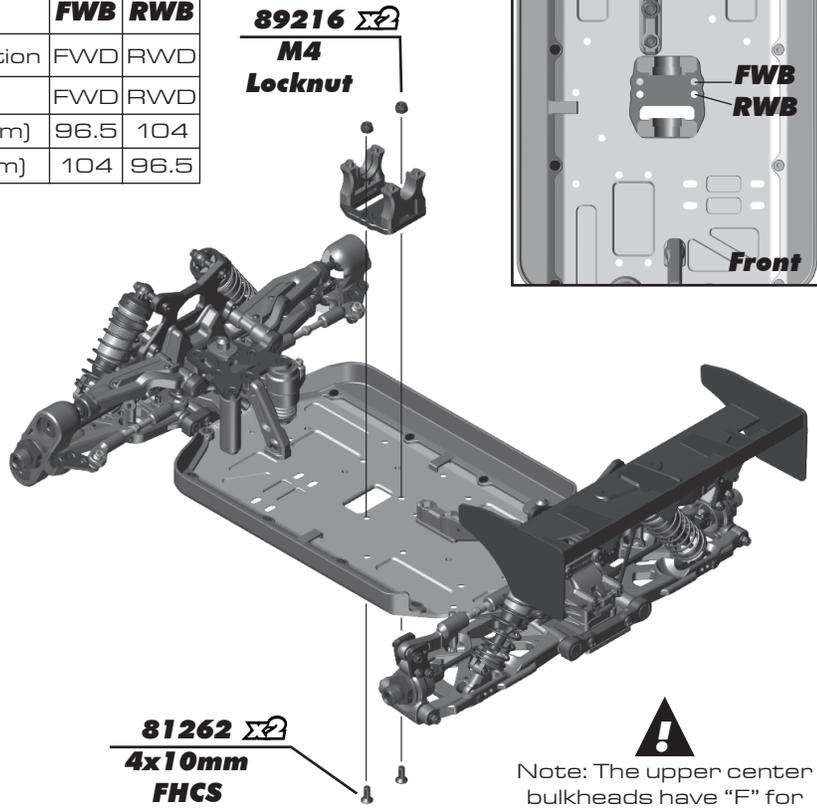
**!** Note: The upper center bulkheads have "F" for front and "R" for rear.
