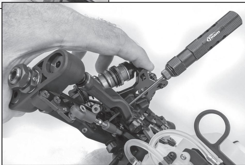
**Front Droop:** Increasing front droop (loosen droop screws) will increase off-throttle steering. It also allows the front end to lift more, giving more rear grip and less front grip on-power. Remember to never loosen the screws beyond the FULL DROOP setting. Decreasing front droop (tighten droop screws) yields more on-power steering and quicker response at the expense of some stability in bumpy sections. It will also give less off-throttle steering.
