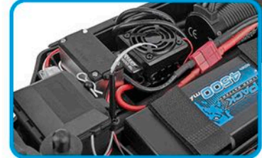
2.4GHz 2-channel radio system with High-Torque Digital Servo and water-resistant, powerful Reedy brushless speed control
