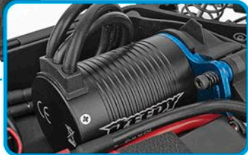
Powerful Reedy 3300kV 4-pole brushless motor
