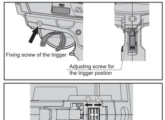
Trigger position gauge Adjustable range: approx. 5mm
