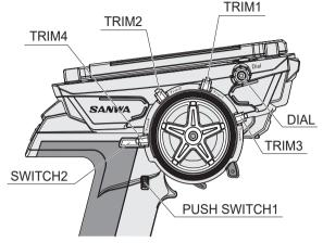
Features assgined to the Switch and Trim at the factory TR1:Steering Trim(TRM-ST) TR2:Throttle Trim(TRM-TH) TR3:Dual Rate ST(D/R-ST) TR4:Dual Rate BR(D/R-BR) SW1:Timer (TIMER) SW2:CUSTOM
