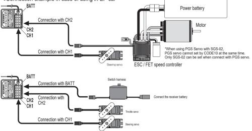
Case of connecting PGS servo and SUPER VORTEX Gen2 / PRO / Stock / SV-D2 to SSL port
