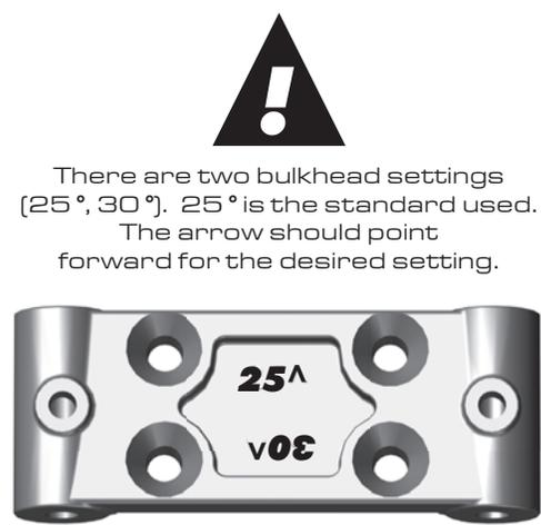
There are two bulkhead settings (25°, 30°). 25° is the standard used. The arrow should point forward for the desired setting.
