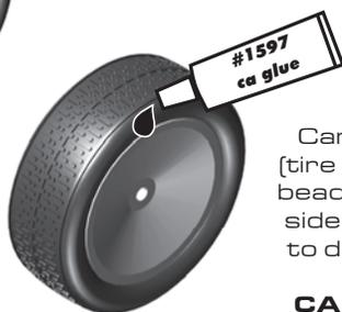
! Carefully apply ca glue (tire adhesive) to the tire bead on the side. Do one side at a time, allowing it to dry before gluing the other side!
