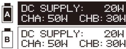
Then, the channel B and DC power supply will take the rest power automatically (For example, if you set DC power supply as 20W and Channel A as 50W, the Channel B will take the rest power of 30W).
