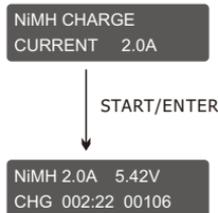
Press the ENTER button and the amp rate value will begin blinking. Use the DEC or INC button to adjust the value to the desired rate. Follow the instructions provided on your battery when setting the charge current.
