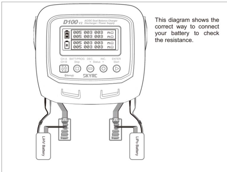
This diagram shows the correct way to connect your battery to check the resistance.
