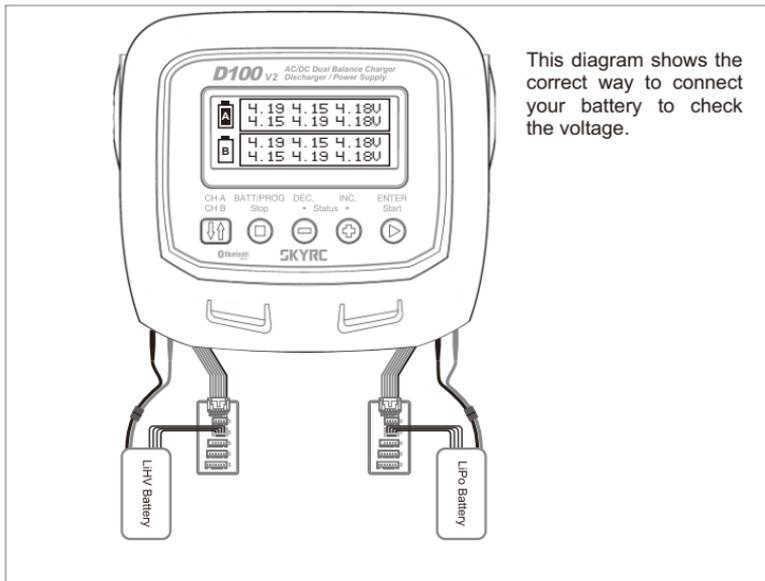
This diagram shows the correct way to connect your battery to check the voltage.
