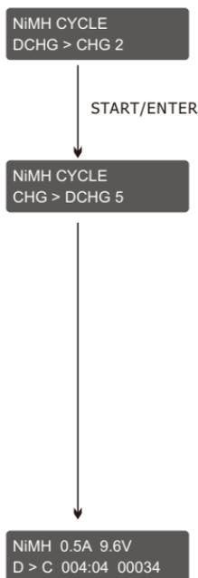
After selecting the correct battery type, use the INC or DEC button to select the “CYCLE” mode. The Cycle Mode gives you two cycling options: “DCHG>CHG” or “CHG>DCHG”. The “DCHG>CHG” option will first discharge the battery and then recharge the battery.
