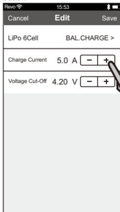
Press to save the program after set the charge current and voltage cut-off
