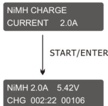
Press the ENTER button and the amp rate value will begin blinking. Use the DEC or INC button to adjust the value to the desired rate. Follow the instructions provided on your battery when setting the charge current. Press and hold the ENTER button for 3 seconds to start charging.
